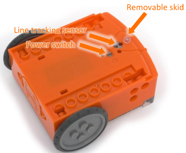
Location of Edison's power switch, skid, and line tracking sensor.
